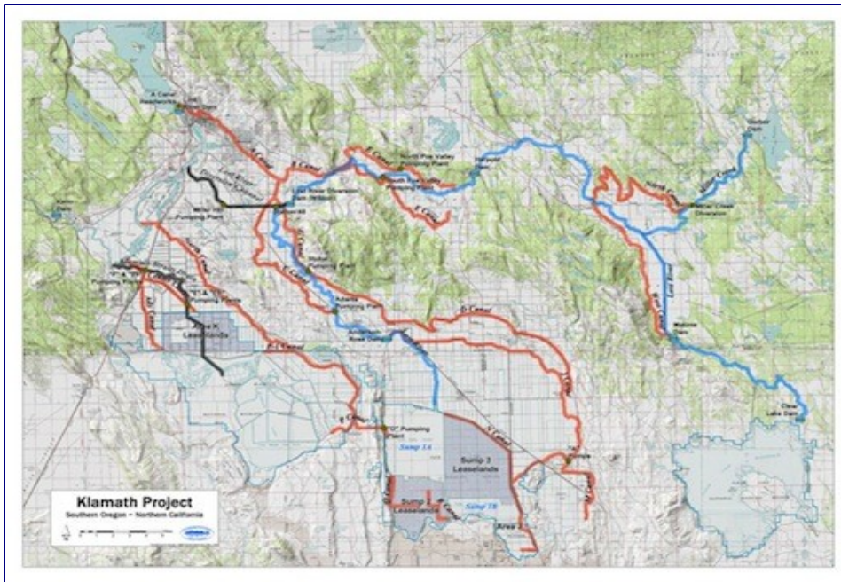
The Klamath Irrigation Project with major canals and pumping plants. There are four national wildlife refuges within the area shown.
